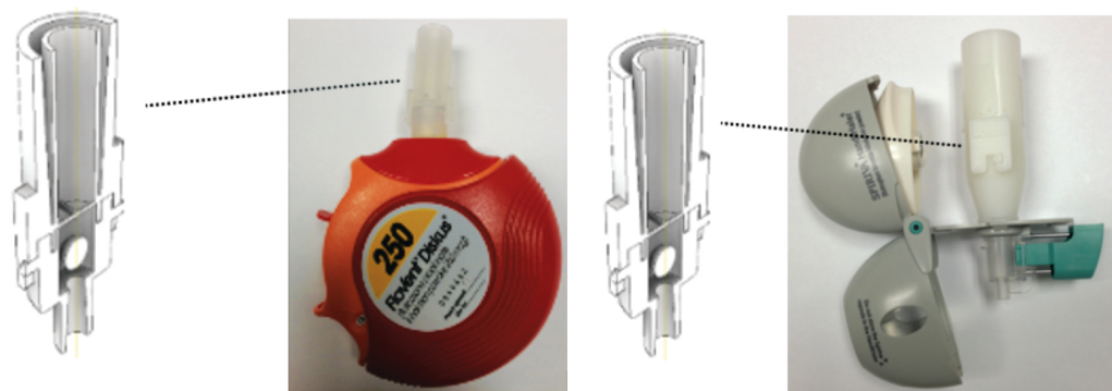
Figure 2. Schematic view of the internal design of the rapid prototyped adaptor (left) used to couple the AOS ™ engine to the commercial Diskus ® device (left) and HandiHaler ® (right). The device was coupled to the outlet of the mouthpiece of the Diskus and capsule chamber of the HandiHaler.
