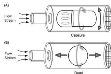
**Fig. 1.** Illustration depicting relative capsule and bead motions in the Handihaler. The polystyrene bead oscillates rapidly near the center of the dispersion chamber, with infrequent contact against the inner walls of the DPI. Though only a single arrow is provided depicting the rotation of the polystyrene carrier, during actuation the bead spins three dimensionally.
