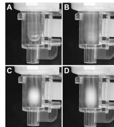
**Fig. 4.** Long exposure photographs of capsule and bead motion. At 15  $\text{L min}^{-1}$  the image of the capsule (A) is not blurred because it remained stationary throughout the 4 second exposure. By contrast, the capsule at 30  $\text{L min}^{-1}$  (B) produced a blurred image as it vibrated rapidly in the dispersion chamber. The polystyrene beads oscillated at both 15  $\text{L min}^{-1}$  (C) and 30  $\text{L min}^{-1}$  (D), though their respective frequencies and amplitudes differed.
