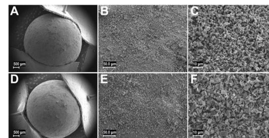
**Fig. 2.** SEM micrographs of polystyrene beads following 2-minutes of piezo-assisted coating with either micronized (A - C) budesonide or (D - F) salbutamol. As seen in figures A and D, the double-sided tape was folded against opposite sides of the polystyrene bead and transfixed to provide adequate conduction for imaging.
